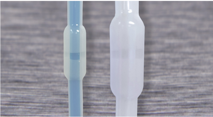
Figure 5: Barb fitting B showing restriction of fluid and hold-up volume at the barb when emptied
