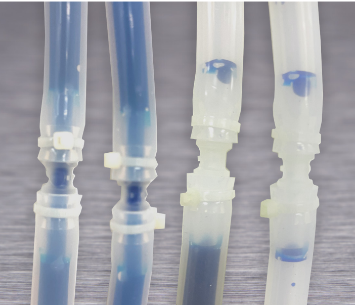
Figure 5: Barb fitting B showing restriction of fluid and hold-up volume at the barb when emptied
