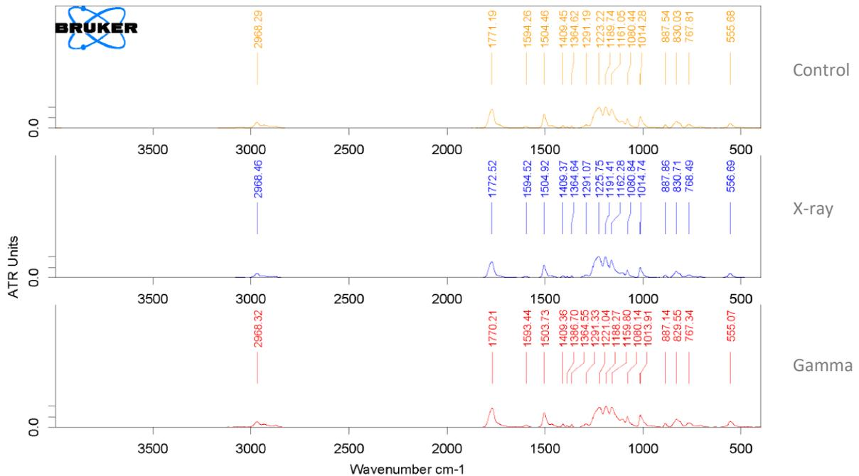
Figure 46: FTIR Spectra of PC used in single use pressure sensors
