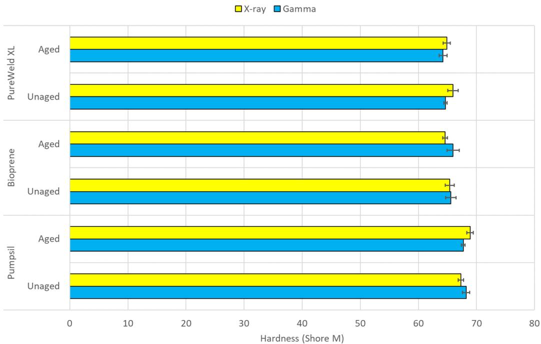
Figure 32: Bar chart of the hardness results in Shore M for unaged, and aged (supplemental) samples. (error bars show one standard deviation).
