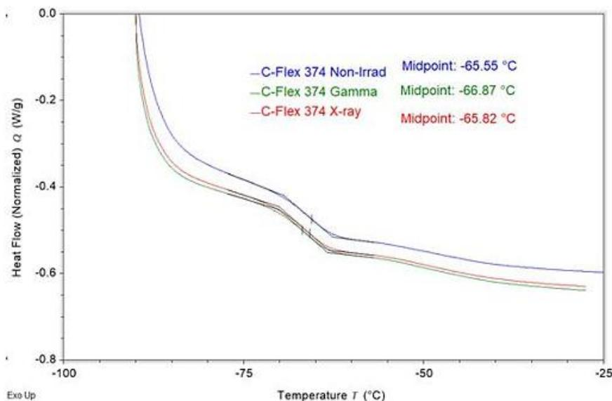
Figure 24: DSC of C-Flex® 374 Tubing
