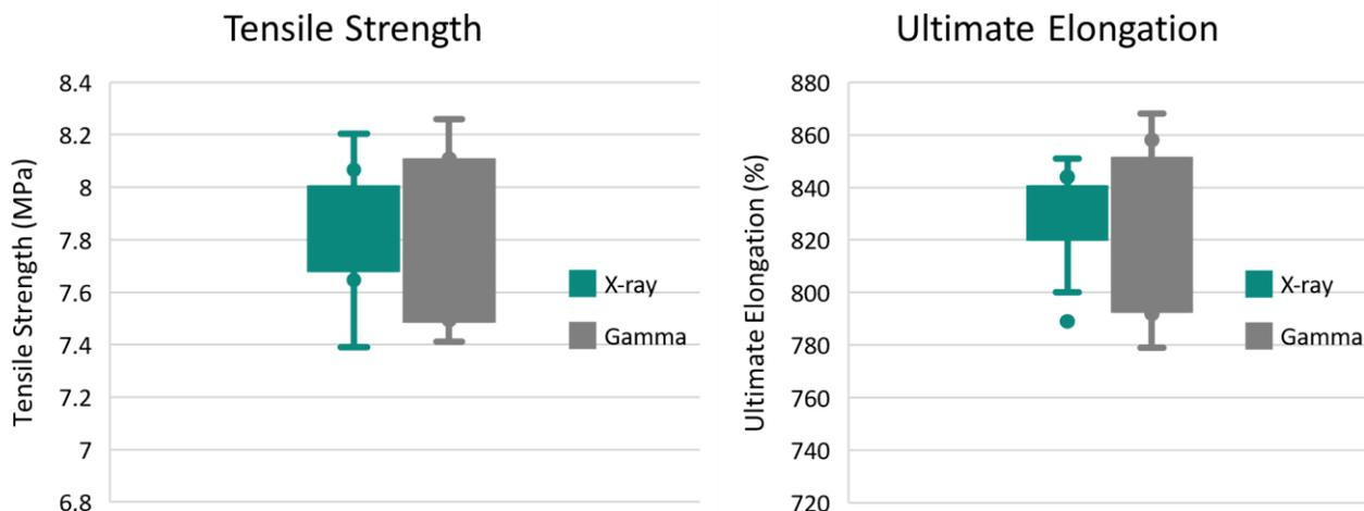
Figure 34: Tensile properties of X-ray (blue) and gamma (orange) irradiated TPE tubing samples.
