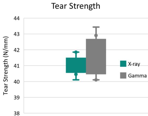
Figure 38: Tear strength properties of X-ray (blue) and gamma (orange) irradiated TPE tubing samples.
