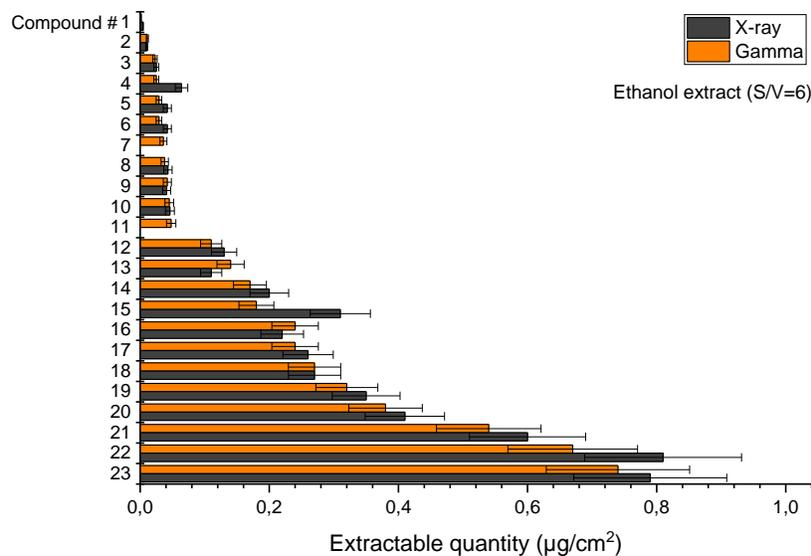
Figure 12: Main outputs of the extractables profile with ethanol extracts on S80 film after Gamma and X-ray, by IC, HPLC-UV, GC-MS and LC-MS
