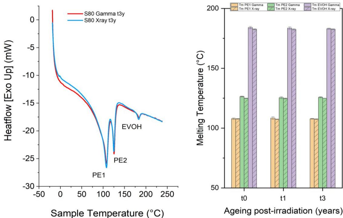
Figure 22: (left) Example of DSC thermograms (2<sup>nd</sup> heating) obtained for the S80 film after gamma and X-ray irradiation. (right) Melting temperatures of the materials of construction of the S80 film (PE1: yellow; PE2: green; EVOH: purple).
