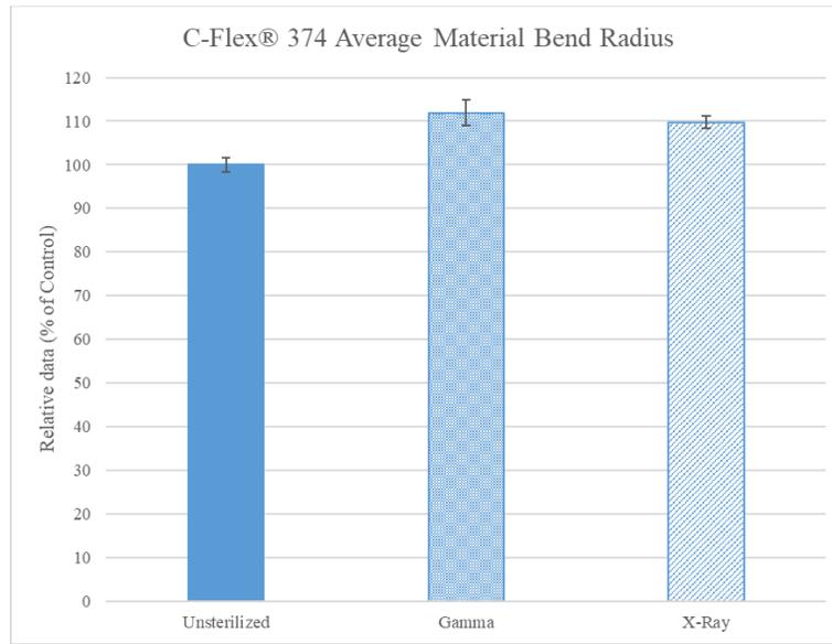
Figure 8: C-Flex® 374 relative average material bend radius results
