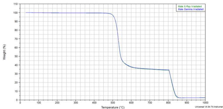
Figure 44: Thermogravimetric analysis of Lynx® S2S (male) connector. Heating 10°C/min
