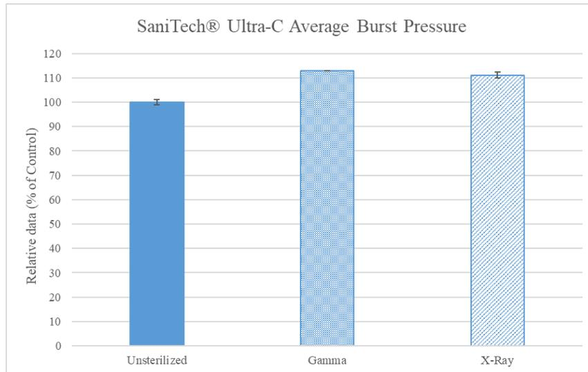
Figure 9: Sani-Tech® Ultra-C relative average burst pressure results
