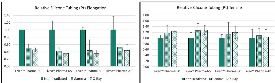
Figure 36: Tensile and elongation at break properties of Liveo™ tubing following irradiation.
