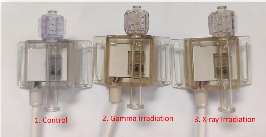
*Figure 15: Control, gamma irradiated, and X-ray irradiated single use pressure sensors*
