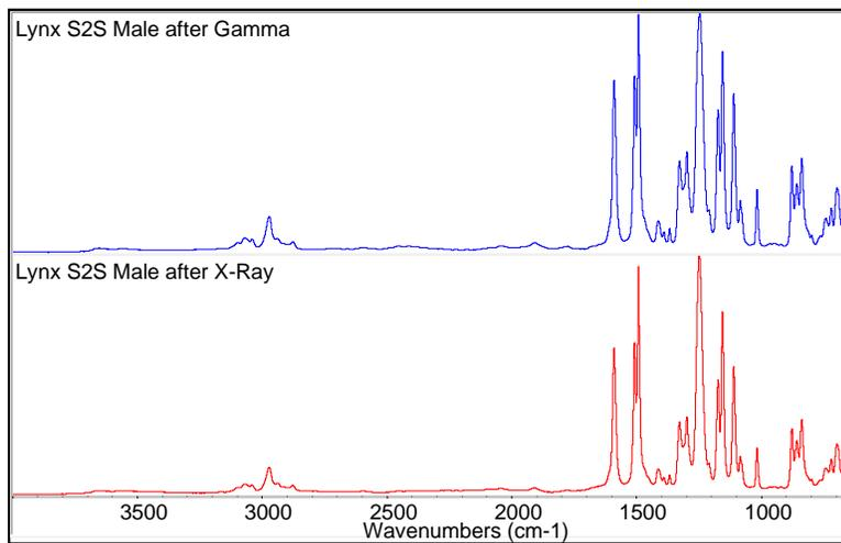
Figure 43: FTIR-ATR spectra on Lynx® S2S connectors (male)
