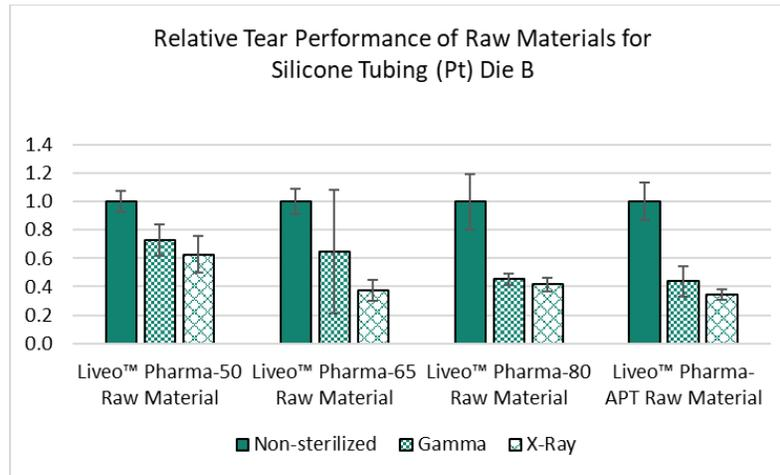
Figure 40: Tear resistance of raw materials for silicone tubing
