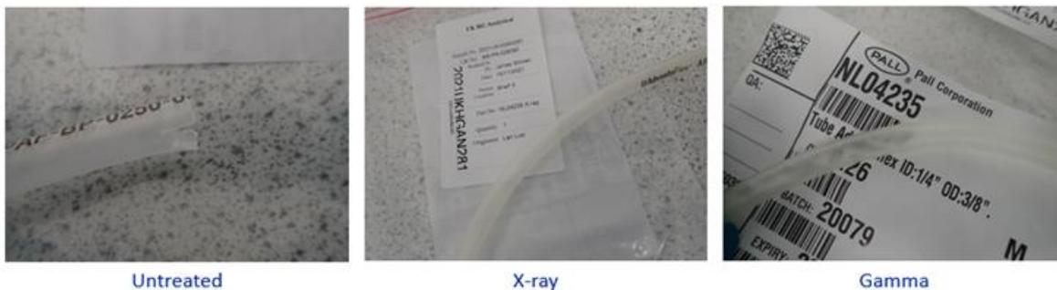
Figure 19: Visual observation and color of the APAF TPE tubing
