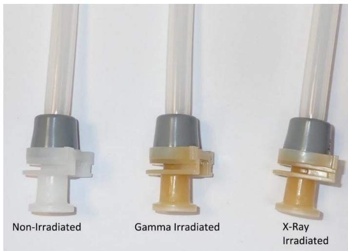
Figure 18: Visual comparison of Pumpsil® LoadSure® connectors.
