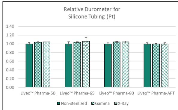
Figure 31: Relative durometer of the Liveo™ Silicone tubing.
