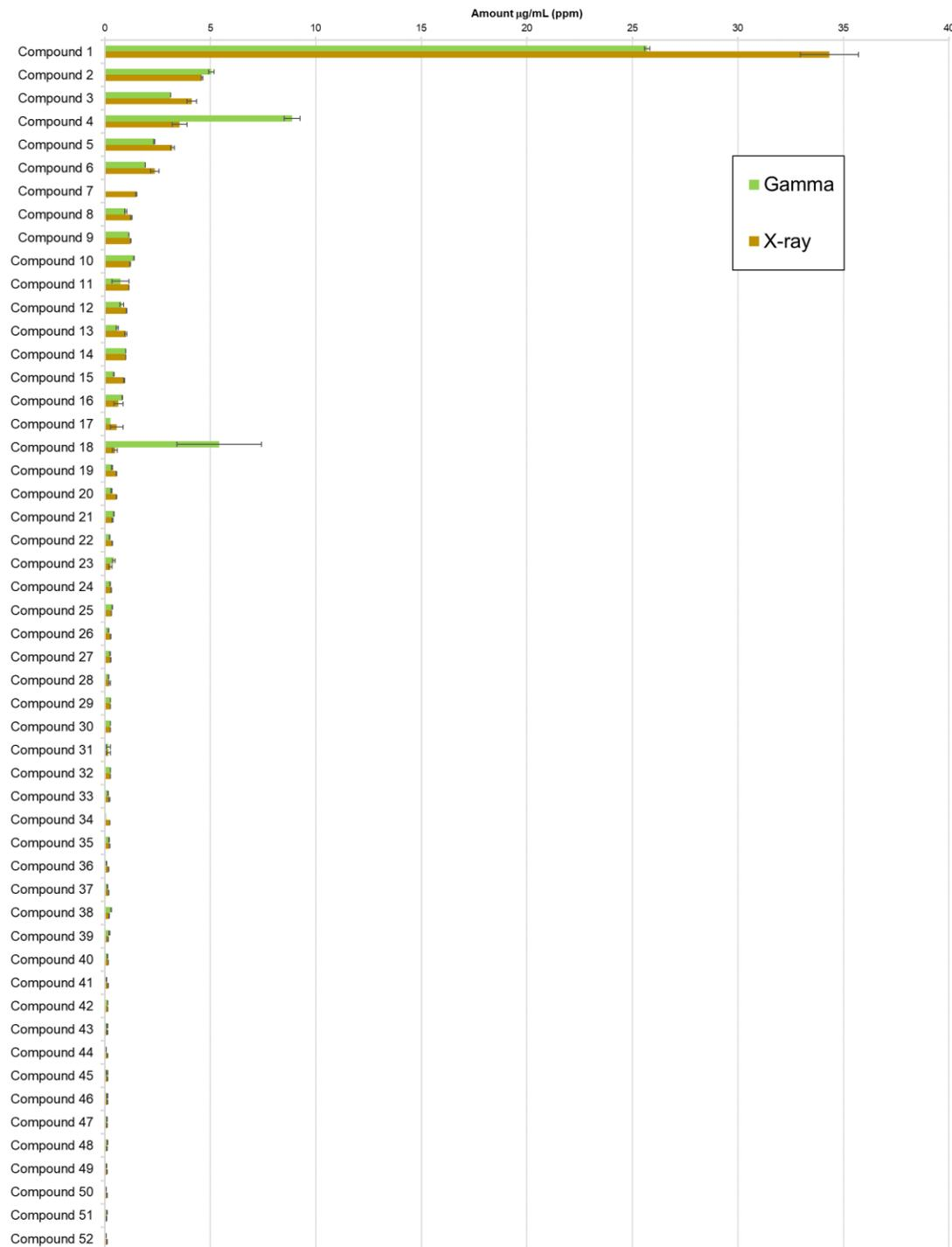
Figure 14: Grand summary of organic extractables (ppm) from gamma irradiated and X-ray irradiated and gamma irradiated APAF TPE tubing. For any values at less than detection or quantitation limit, respective limits are shown.
