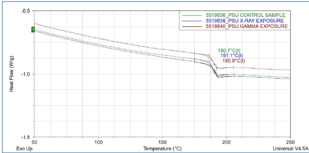
Figure 45: DSC thermograms of polysulfone sensor material: control, gamma and X-ray irradiated
