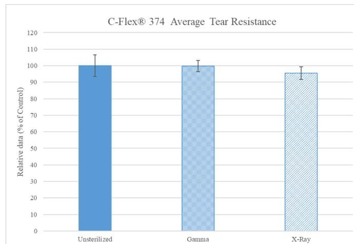
Figure 39: C-Flex® 374 relative average tear resistance results
