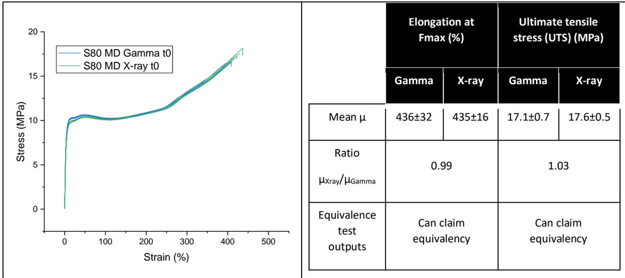
Figure 33: (left) Stress-strain curves for S80 film in machine direction (MD) (t0) – (right) Elongation at Fmax and ultimate tensile stress (UTS) results
