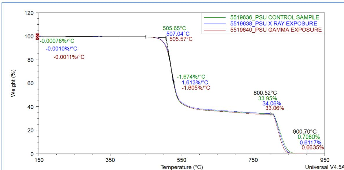
Figure 29: TGA curves of PSU sensor material
