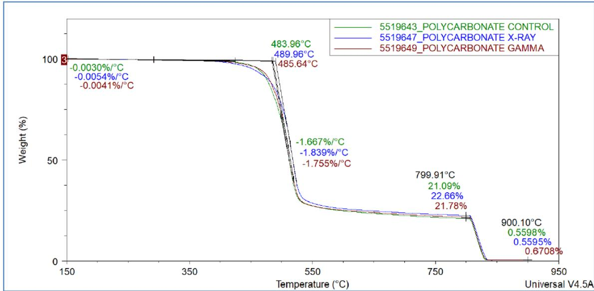
Figure 47: Thermogravimetric analysis of polycarbonate materials in PendoTECH sensor.
