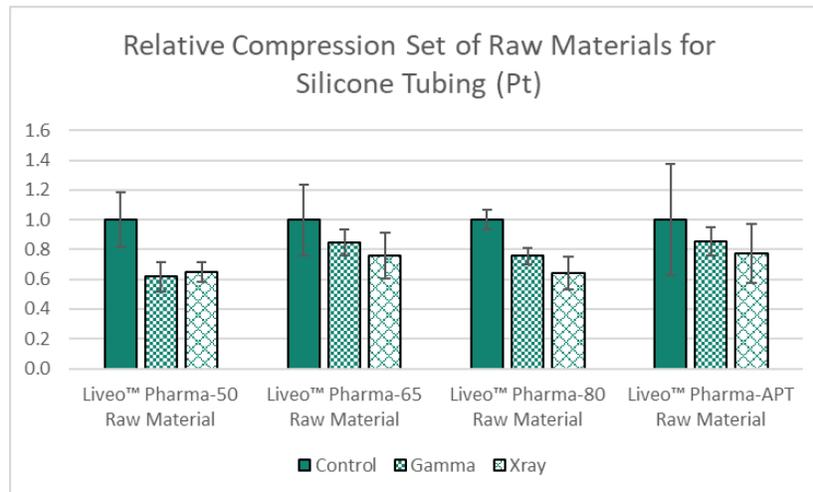
Figure 42: Compression set testing of Liveo tubing materials
