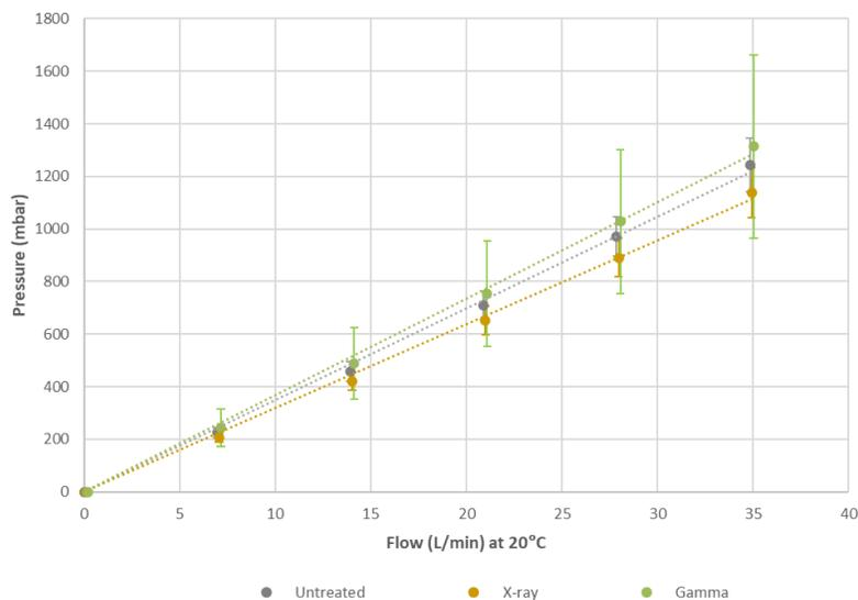
Figure 2: Water flow vs. differential pressure test results for untreated (black), gamma irradiated (green), and X-ray irradiated (gold) KA3EKVP1 filter capsules
