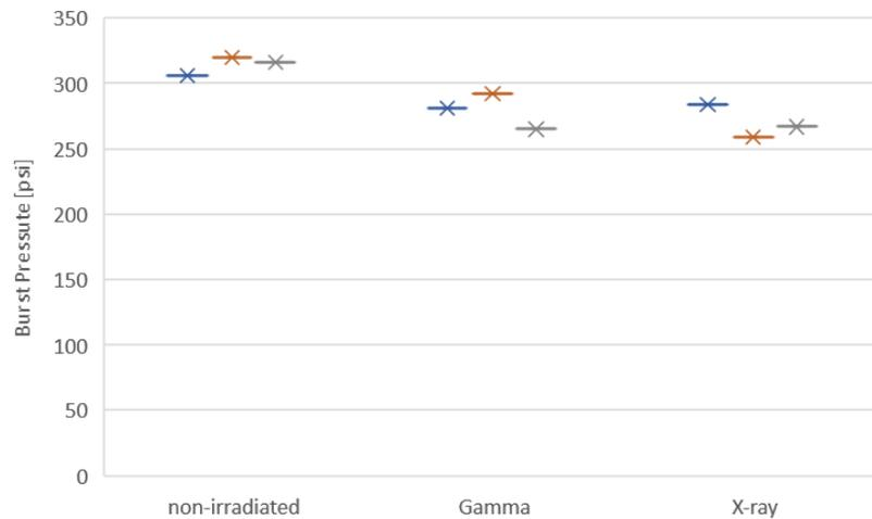
Figure 1: Pressure burst test results for untreated, gamma irradiated, and X-ray irradiated Kleenpak™ filter capsules
