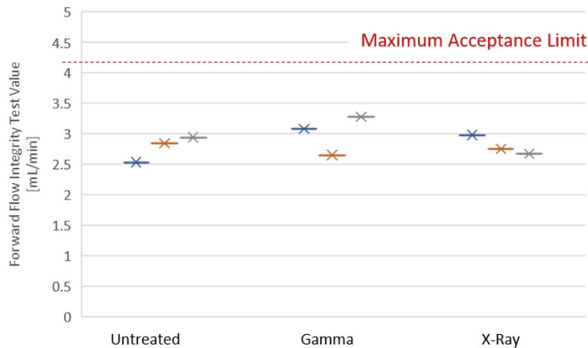
Figure 3: Forward flow filter integrity test results for untreated, gamma irradiated, and X-ray irradiated KA3EKVP1G filter capsules wetted with water.
