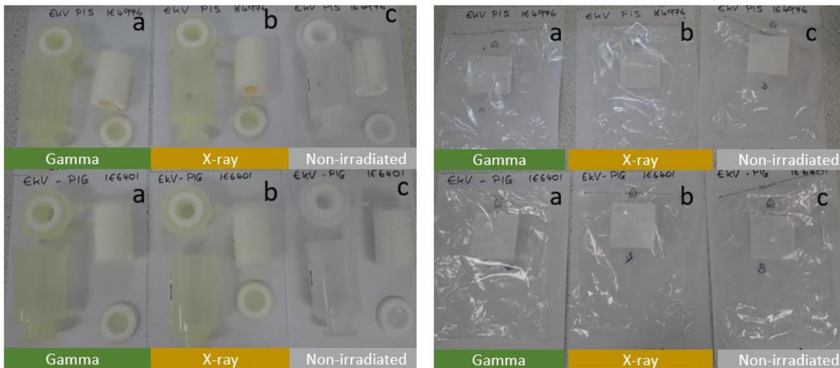
Figure 17: Visual inspection of (left) sectioned KA3EKVP1G filter capsules and (right) component packaging materials
