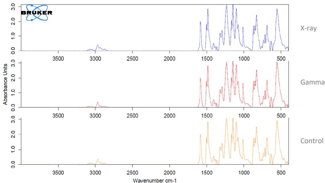
Figure 25: FTIR Spectra of PSU used in single use pressure sensors
