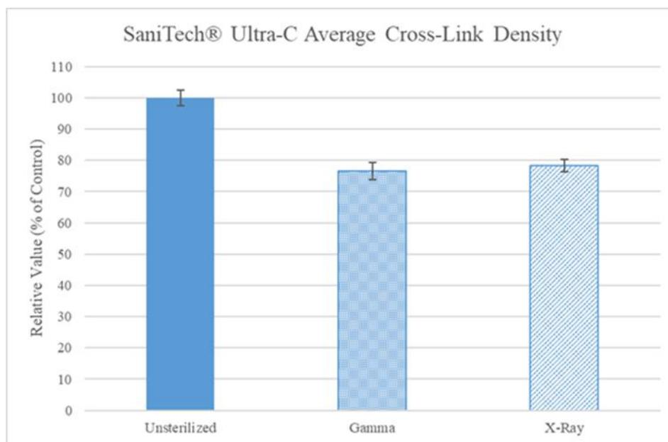
Figure 37: Sani-Tech® Ultra-C relative average cross-link density
