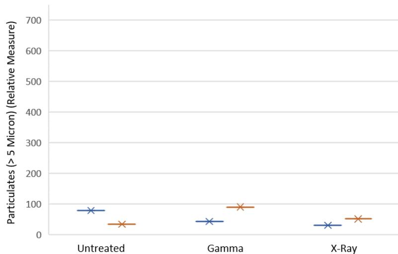
Figure 48: Particulate levels (> 5 micron) in filter effluent evaluated without prior flushing evaluated for non-irradiated, gamma irradiated, and X-ray irradiated filter capsules
