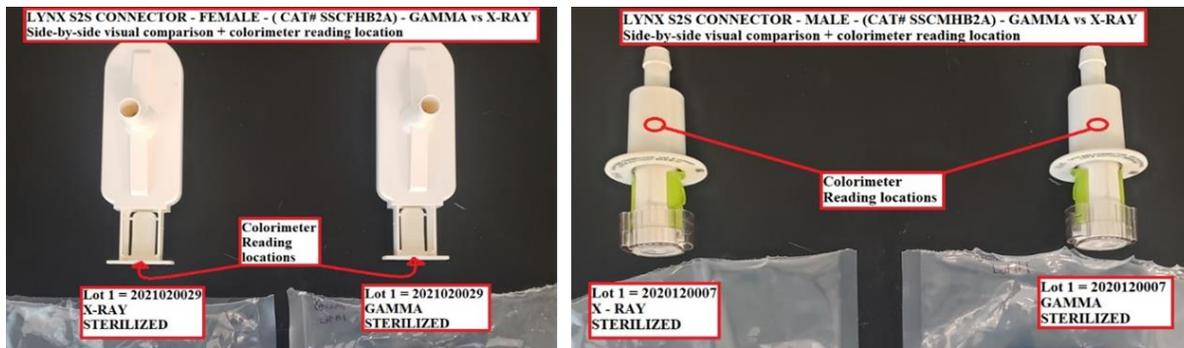
Figure 16: Lynx® male and female S2S connector post gamma & post X-ray
