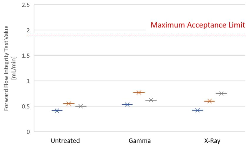
Figure 49: Forward flow test results for untreated, gamma irradiated, and X-ray irradiated KA3EKVPG1 filter capsules wetted with 60/40 IPA/water
