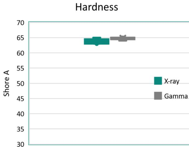
Figure 30: Hardness (Shore A) properties of X-ray (blue) and gamma (orange) irradiated TPE tubing samples.
