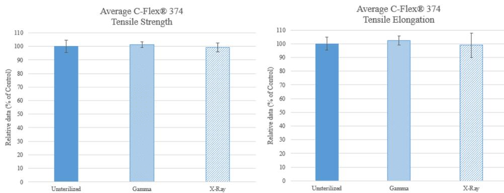
Figure 35: C-Flex® 374 Tensile Strength and Elongation
