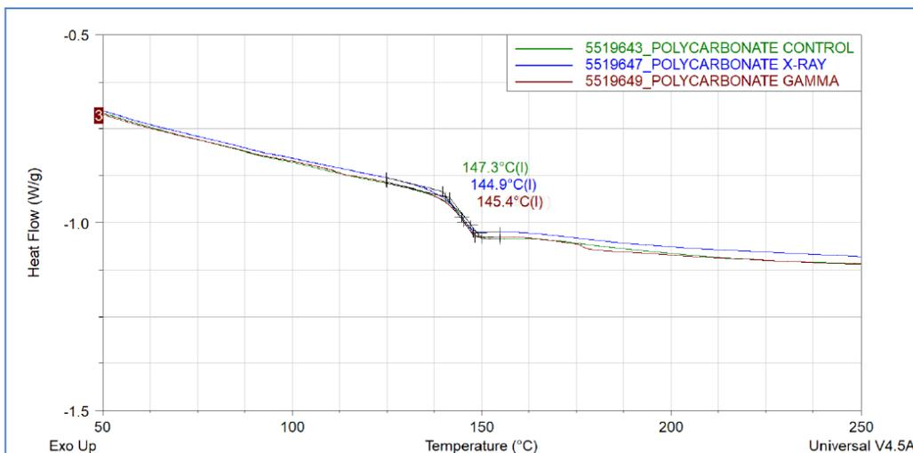
Figure 21: DSC thermograms of polycarbonate sensor material: control, gamma and X-ray irradiated
