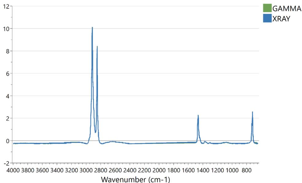
Figure 26: ATR-FTIR spectra for S80 film after AsLS (asymmetric least squares) baseline correction and SNV (Standard Normal Variate) normalization
