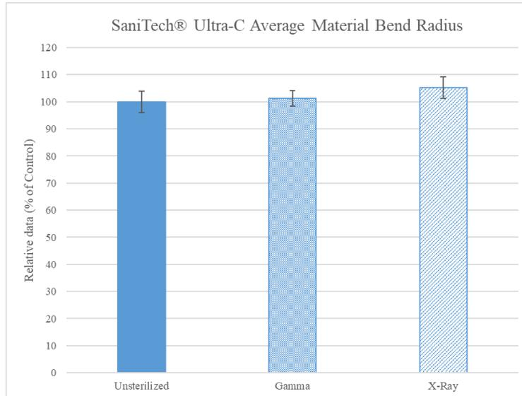
Figure 10: SaniTech® Ultra-C relative average bend radius results
