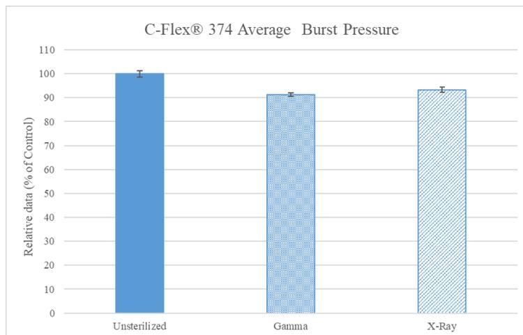
Figure 7: C-Flex® 374 relative average burst pressure results
