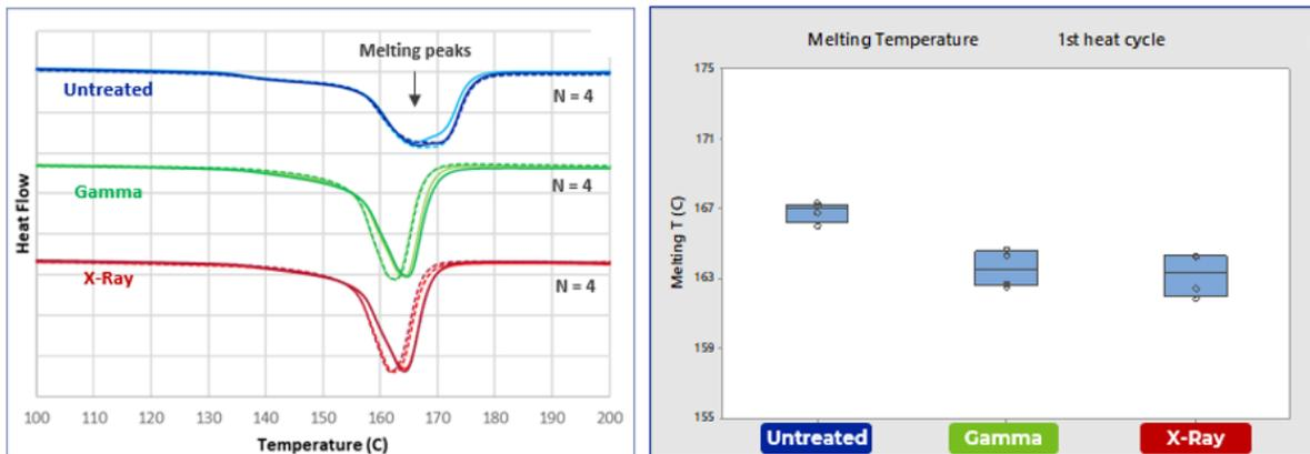
Figure 23: (left) First heating DSC curve for polypropylene filter support material for untreated (blue), gamma (green) and X-ray (red). Melting temperatures. (right) melting temperatures
