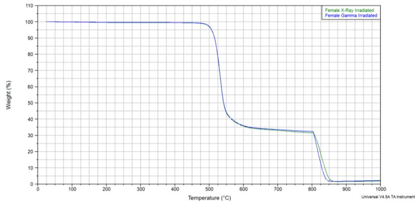
Figure 28: Thermogravimetric analysis of Lynx® S2S (female) connector. Heating 10 C/min.
