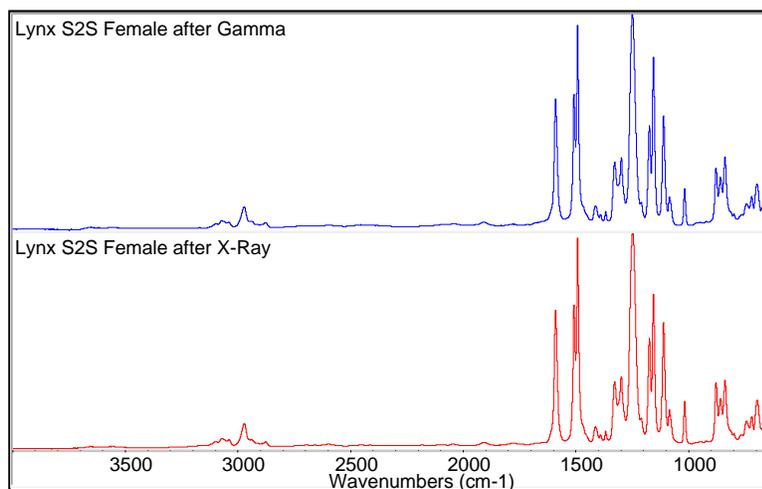
Figure 27: ATR-FTIR spectra on Lynx® connectors (female)
