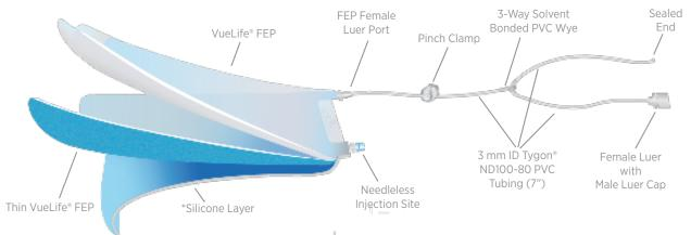
\*Silicone side must face down. Rack required (do not lay on incubator shelf)
