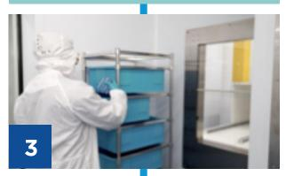
Assembly occurs in ISO 7 cleanroom or in an ISO 5 hood. Assembly could include, but is not limited to: laser welding, gluing, and integrity testing.
