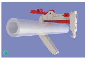
Push Lower-Member to the desired position ("Flow" or "Stop Flow").
