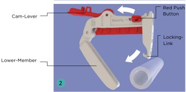
Position the tube in the gate, as close as possible to the hinge of the clamp.
