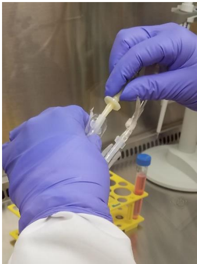
Fig. 8b Insertion of male spike into female spike port
