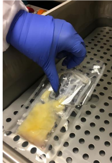
Fig. 6 KryoSure® Bag being placed in water bath
