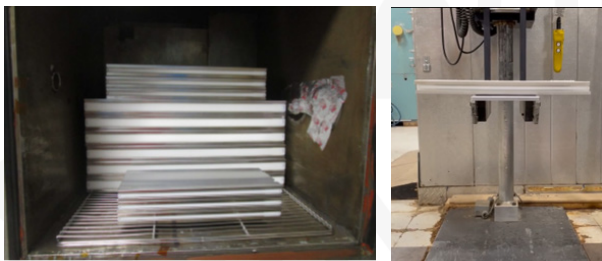
Figure 4. Representative pictures from conditioning and drop test setup. Left image shows conditioning chamber and right image shows drop tester.
