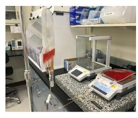
Figure 2. Addition of culture media from media bag to VueLife® culture bag. Bag contents can be transferred via gravity and volume can be tracked by using a lab scale.
