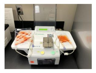
Figure 3. VueLife® bags can be connected using a sterile connection device and welding the ends of the Y-tubing.
